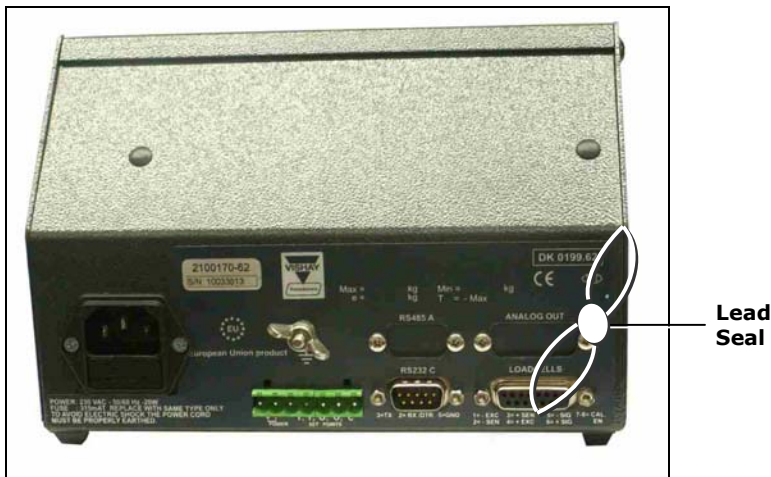
Figure 11 – Desktop model, sealing with lead seal / non-removable sticker
